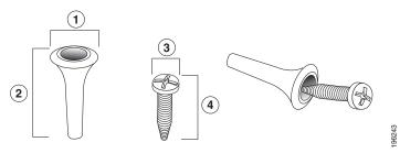
1 8 mm/0.4 in 2 22.2 mm/0.9 in 3 6.8 mm/0.3 in 4 17.6 mm/0.7 in
